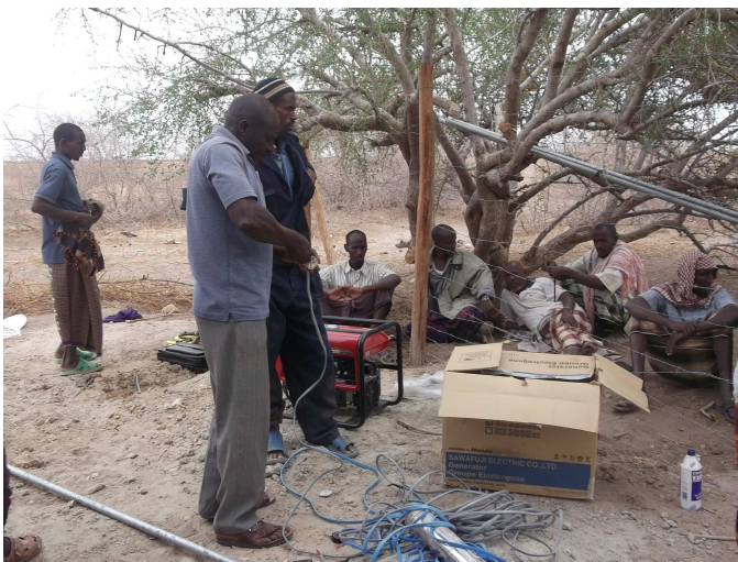
Technicians preparing for the well water yield test
